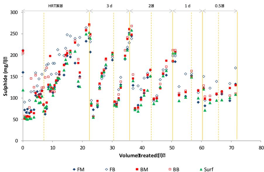
**Figure 3** Aqueous sulphide concentration at different points in the reactor as a function of HRT. Dashed vertical lines indicate biofilm collapse, while complete vertical lines indicate biofilm harvesting
