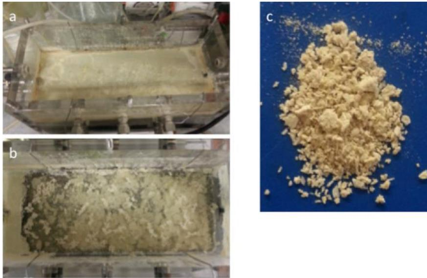
**Figure 2** Photographs showing (a) complete biofilm prior to collapse, (b) the biofilm following collapse onto the submerged screen and (c) the dried sulphur product
