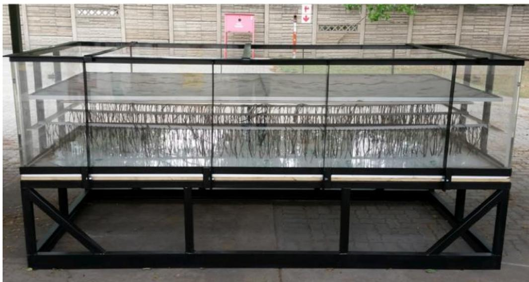
*Figure 1 Image illustrating the pilot scale LFCR reactor on site, prior to inoculation*
