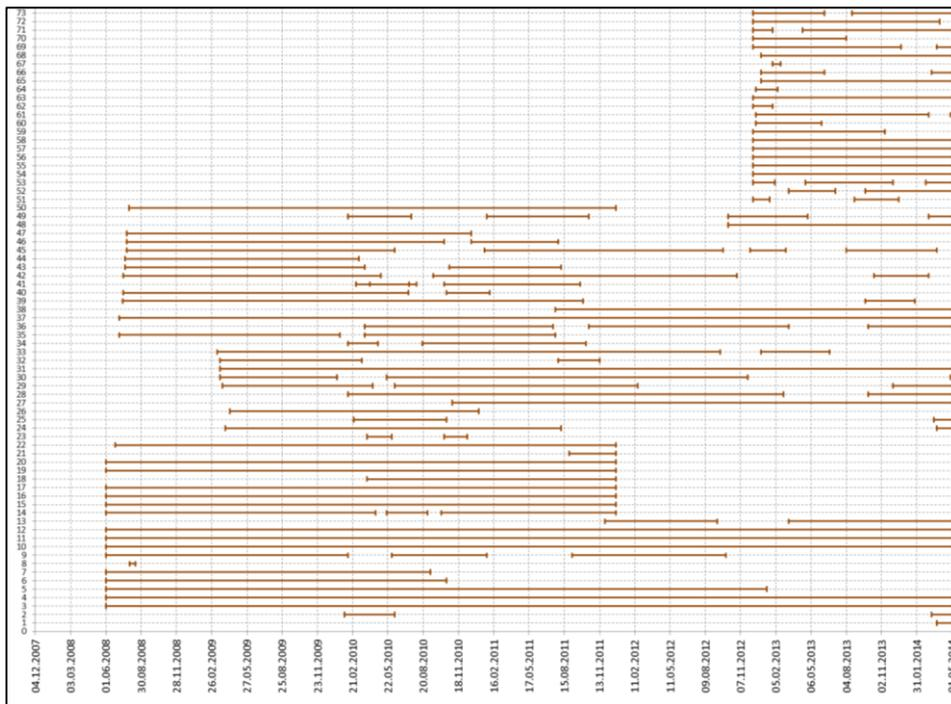
**Figure 4:** Pumping schedule of the shallow dewatering wells.
