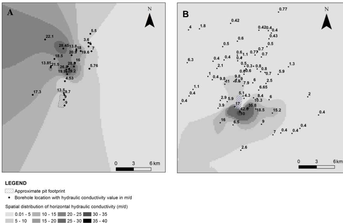
Figure 1: Spatial distribution of hydraulic conductivity of shallow aquifer (A) and deep aquifer (B)
