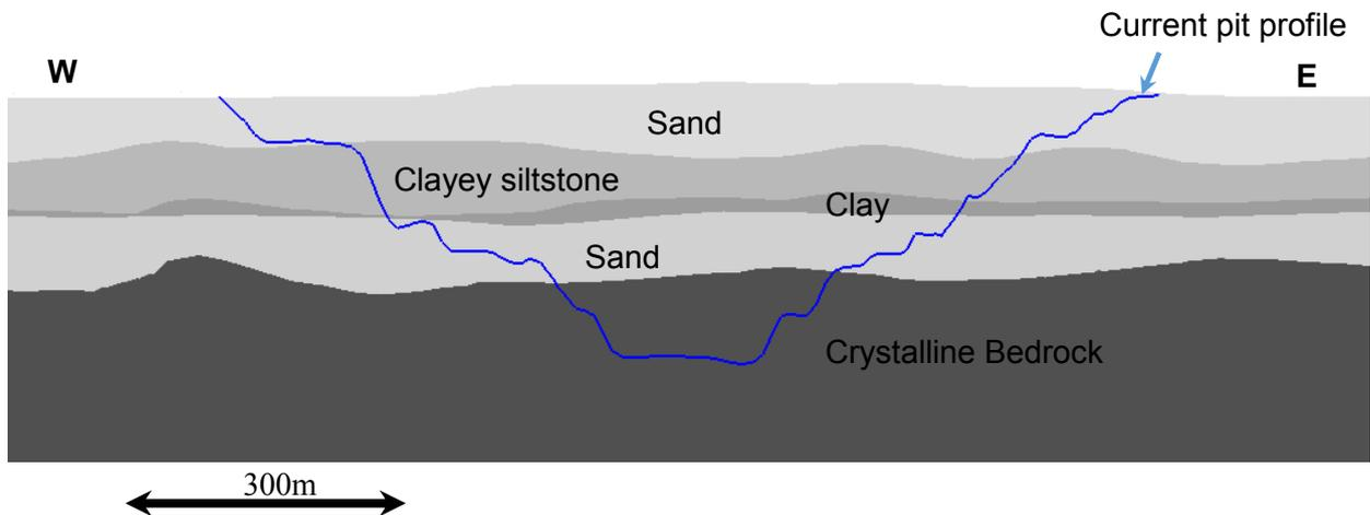
Figure 2: East-West geological section across the pit (vertical exaggeration: 3x)
