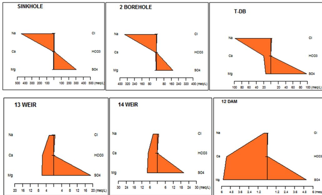
**Figure 3:** Stiff diagram for samples collected from the sinkhole, borehole and T&DB which are classified as having Na-SO<sub>4</sub> type of water.
