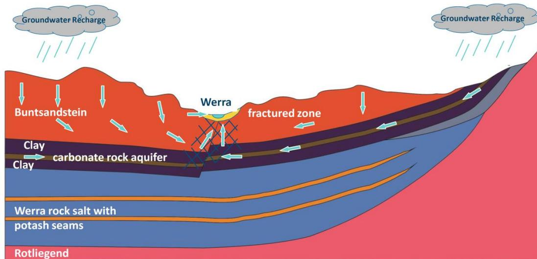
**Figure 2** Schematic hydrogeological situation in Werra potash mining region.
