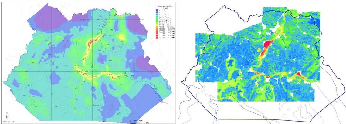
Figure 6 Comparison of the distribution of simulated TDS near to surface (left) with results of measured airborne electrical resistivity (right), where red color indicates comparable high TDS concentrations or high conductivity, respectively.
