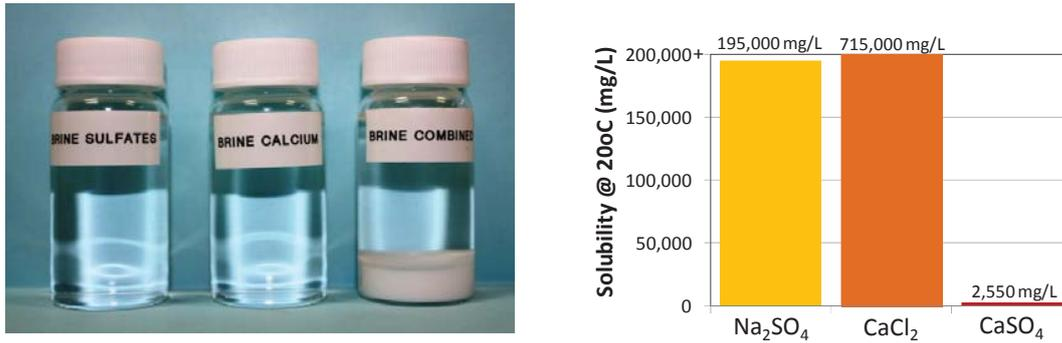
Figure 3: Solubility Limits of  $\text{CaCl}_2$  and  $\text{Na}_2\text{SO}_4$  Solutions
