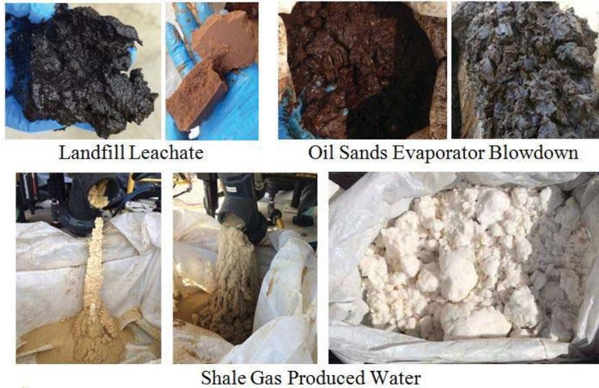
**Figure 8: Low Temperature Crystallizer True ZLD Solids**
