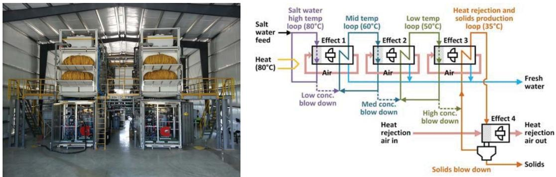
Figure 4: 100 m<sup>3</sup>/day Low Temperature Crystallizer (left) and Simplified PFD (right)
