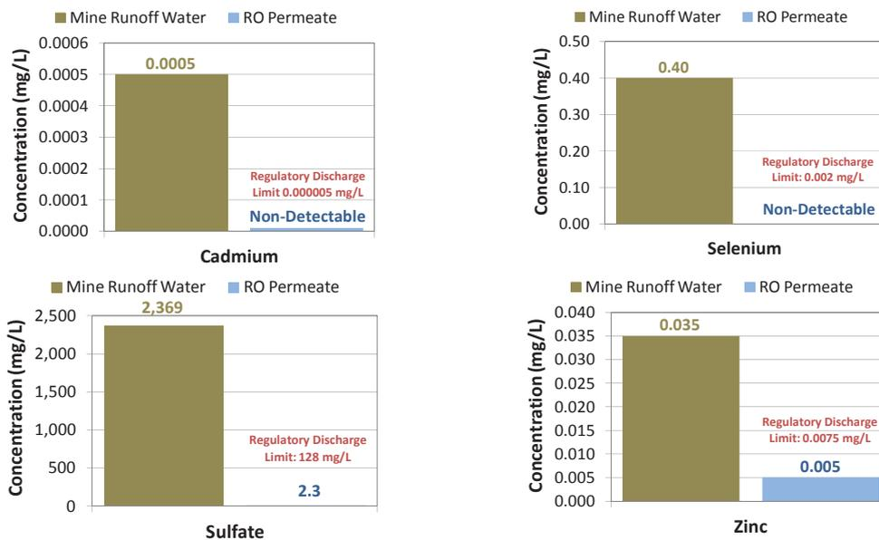
**Figure 7: RO Permeate Water Chemistry Compared to Regulatory Discharge Limits**
