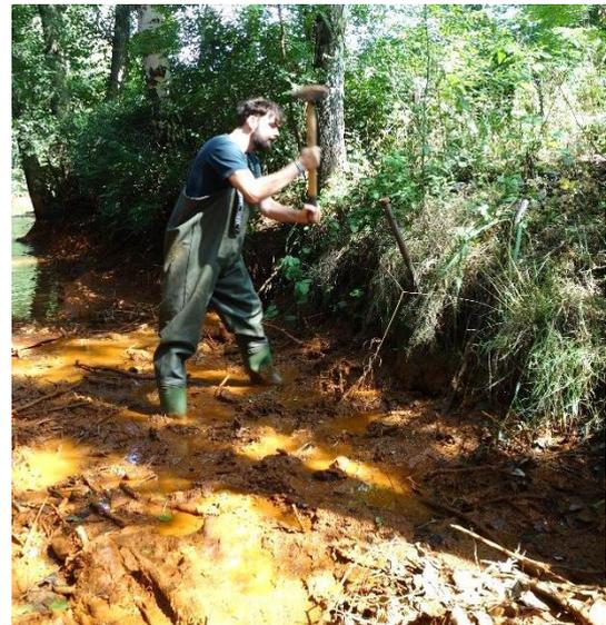
**Figure 4** Typical ramming installation of the WaSP on the bank at sampling point (b), using a hammer.
