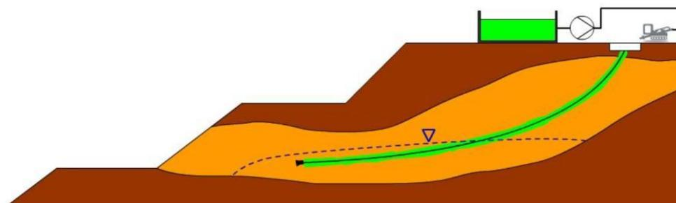
**Figure 3** Scheme Horizontal Directional Drilling (Harzer (2012))
