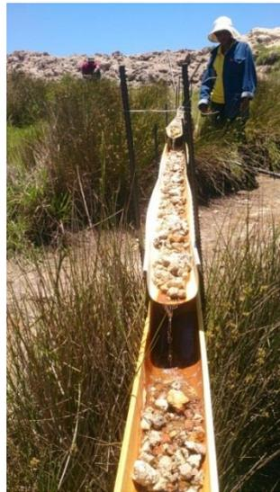
*Figure 3 Carolina pilot passive treatment cascading trench*
