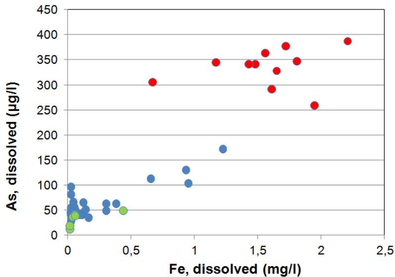
**Figure 7** Correlation of dissolved iron and arsenic concentrations in reaction cell effluents (m-241P) during test periods 2c (baseline monitoring prior to H<sub>2</sub>O<sub>2</sub> dosage, red dots), 4-5 (H<sub>2</sub>O<sub>2</sub> dosage, blue dots) and 6 (H<sub>2</sub>O<sub>2</sub> dosage, green dots)
