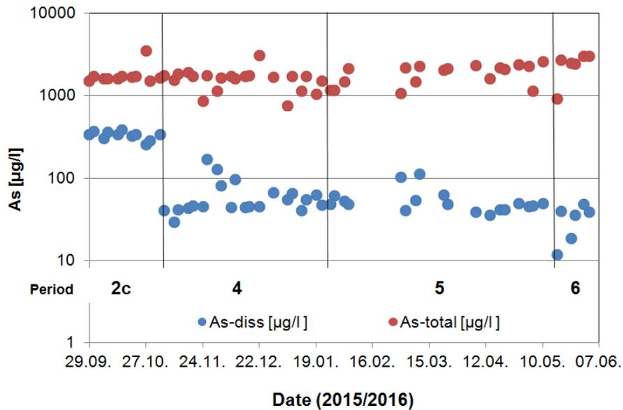
**Figure 6** Total and dissolved arsenic concentrations in reaction cell effluents (prior to filtration, m-241P) during test periods 2c (baseline monitoring prior to H<sub>2</sub>O<sub>2</sub> dosage) and 4-6 (H<sub>2</sub>O<sub>2</sub> dosage)
