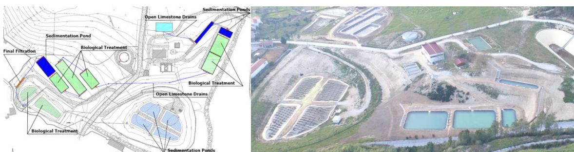
Figure 10 Cunha Baixa passive treatment process and photo.
