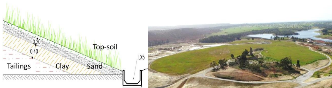
Figure 5 Clay cover system in Aljustrel old mining area and photography after remediation works.
