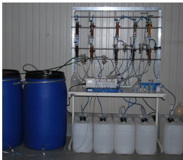
Figure 3 Pilot test setup: influent 200L-influent barrels, columns, peristaltic pump and effluent canisters
