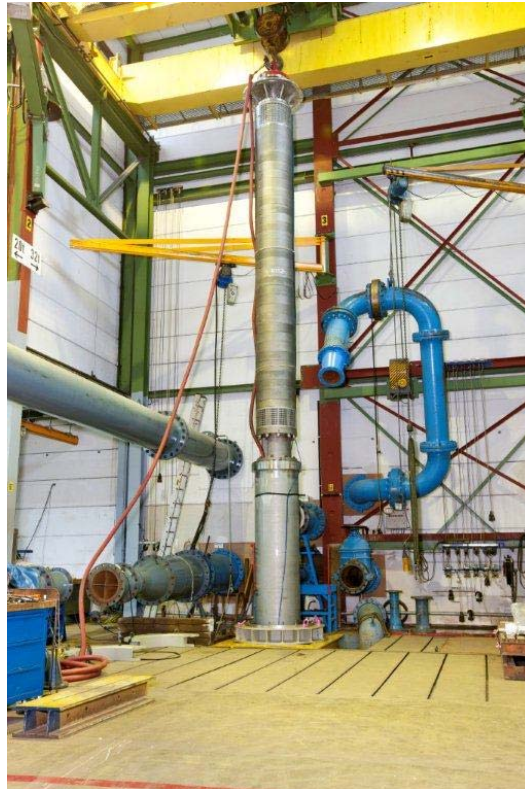
Figure 1: A Ritz HMD pump being placed in the test bay. Note the two suctions to combat axial thrust.
