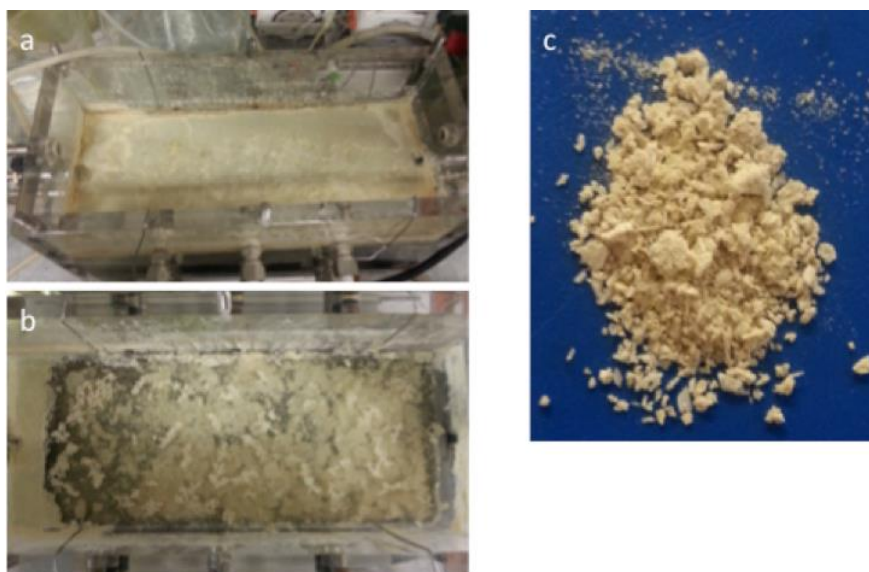
Figure 2 Photographs showing (a) complete biofilm prior to collapse, (b) the biofilm following collapse onto the submerged screen and (c) the dried sulphur product
