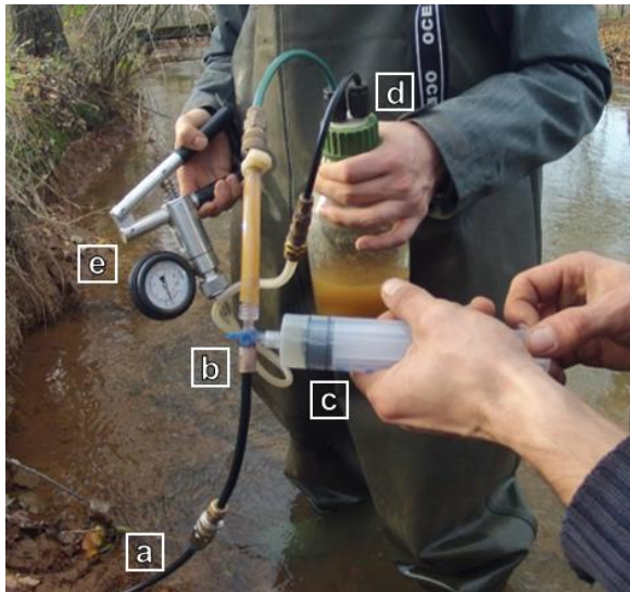
Figure 5 Sampling equipment with the tube from the WaSP (a), a three-way valve (b), the connection to the sampling syringe (c) and the air-tight collection bottle (d) with the vacuum pump (e).
