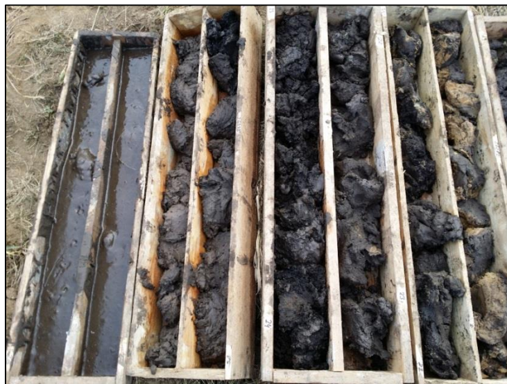
Figure 2: Drill core with muddy (left) to semi-solid (right) material from Bösau dump.
