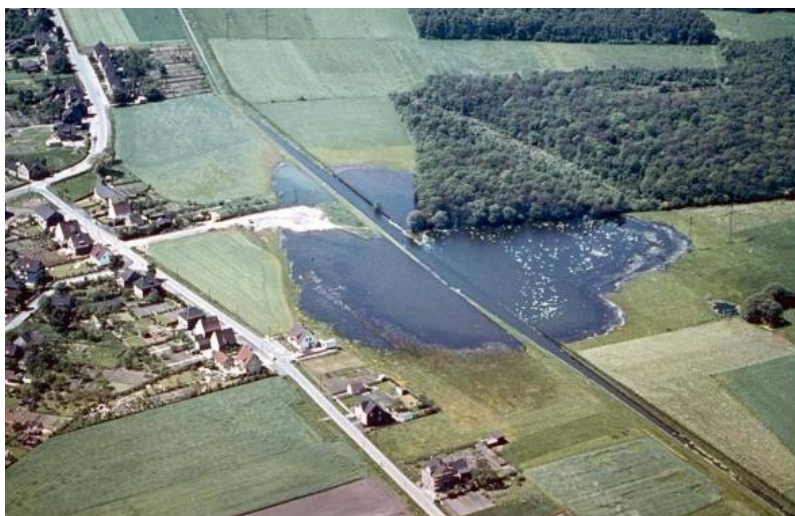
Figure 5 Water logging caused by land subsidence in the German Ruhr coal area.
