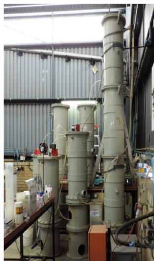
Figure 2 Multi-stage column system used for test work
