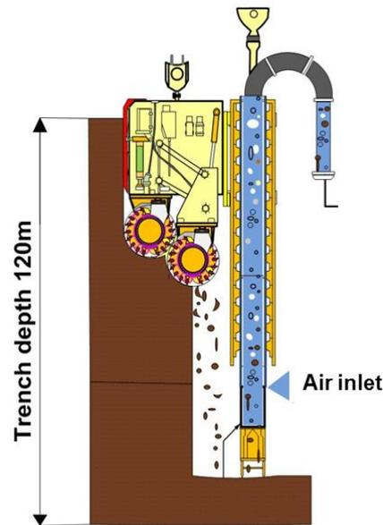
*Figure 4: Guide pile and Cutter BCV 40*
