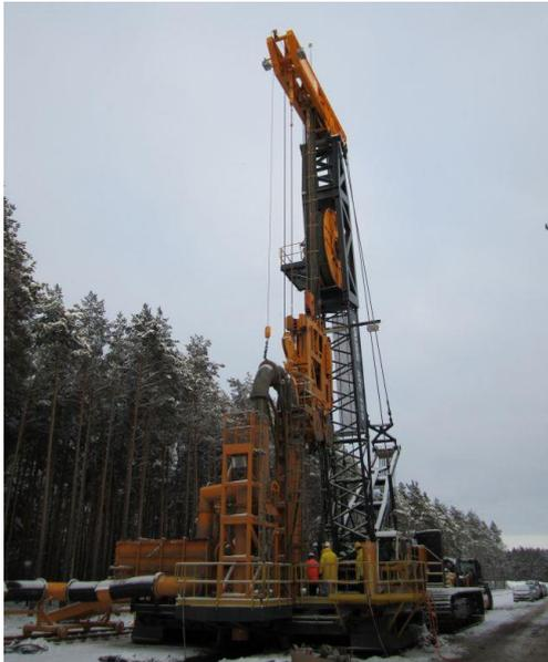
*Figure 3: BAUER BCV 40 – 130 on MC 128*
