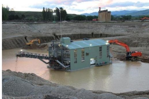
**Figure18:** *Floating recovery plant*
