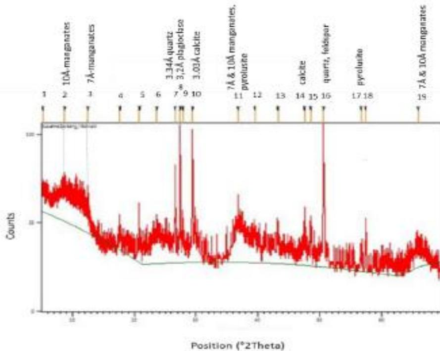
Figure 3 X-ray diffractogram of the precipitate (Sjöberg 2014)
