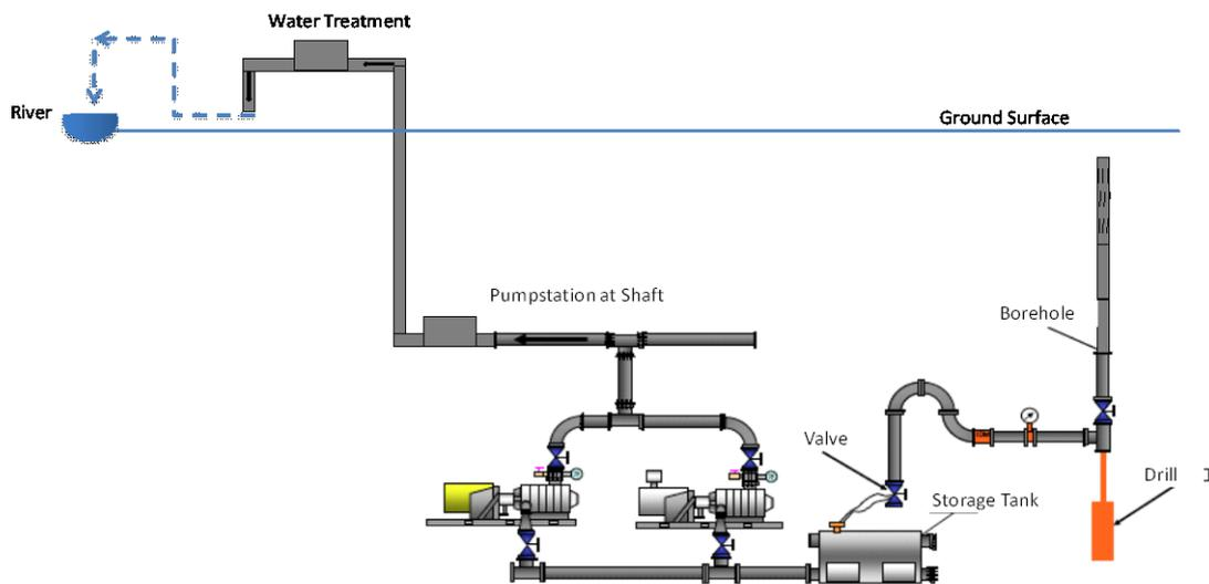
*Figure 3 Dewatering scheme to manage stagnant water in a RAG mine.*
