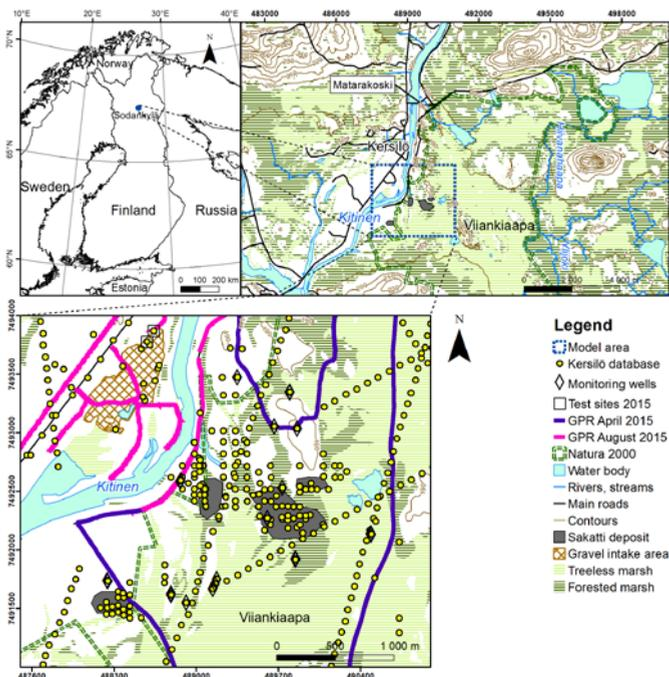
**Figure 1** Location of the study area around the River Kitinen in Northern Finland (above). The Kersilö database and ground penetrating radar (GPR) profiles were used as input data for the 3D model (below). The Kersilö database indicates the locations of available surficial deposit and bedrock surface observations. Terrain polygons © National Land Survey of Finland, Sakatti deposit modified after Brownscombe (2015).
