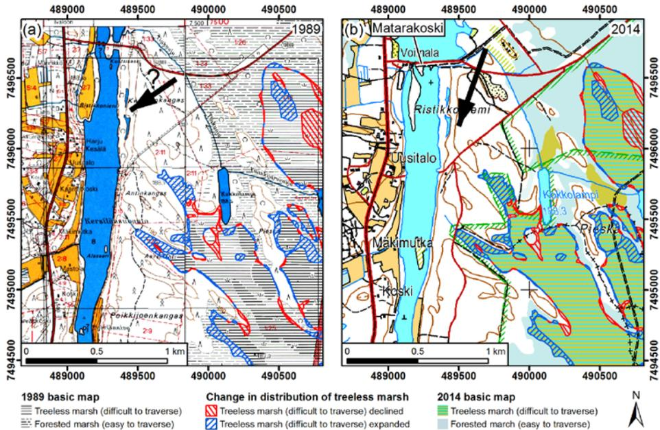
**Figure 4** The change in the distribution of treeless marsh in the Kokkolampi area near Matarakoski hydroelectric power plant. (a) The situation in 1989 before the construction of the Matarakoski hydroelectric power plant; (b) the present situation. The treeless marsh area increased near Kokkolampi from 1989 to 2014. The black arrows indicate the estimated groundwater flow directions near Matarakoski. Basic maps (2014, 1989) © National Land Survey of Finland.
