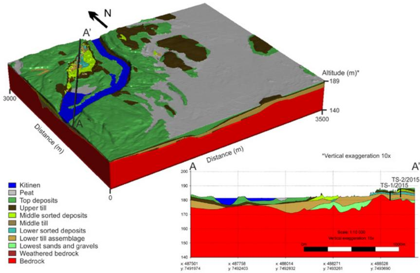
**Figure 2** 3D model of unconsolidated sediments and bedrock topography near Kersilö village (above) and cross-section A-A' of the 3D model (below). The location of the 3D model is presented in fig. 1. The sediment structure is tentatively based on the interpretation of the test sites TS-1/2015 and TS-2/2015.
