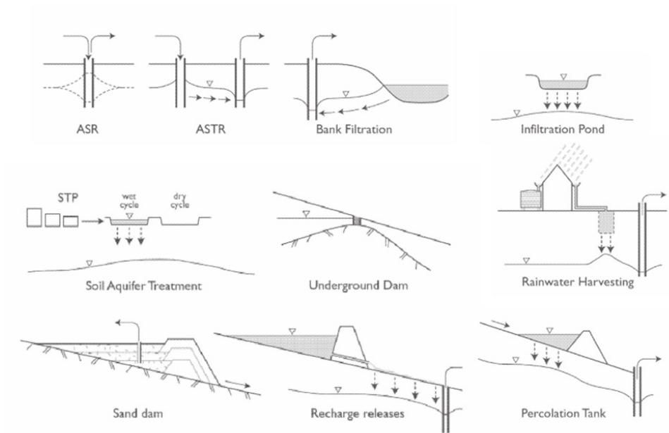
**Figure 3** Schematic of types of management of aquifer recharge (Dillon, 2005). Abbreviations: ASR=Aquifer Storage & Recovery, ASTR=Aquifer, Storage, Transfer & Recovery, STP = Sewage Treatment Plant.
