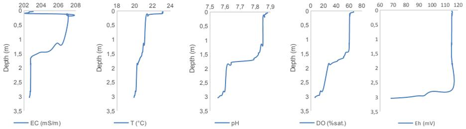
Figure 13: Water column profiles of Pit lake D (March 2017.)
