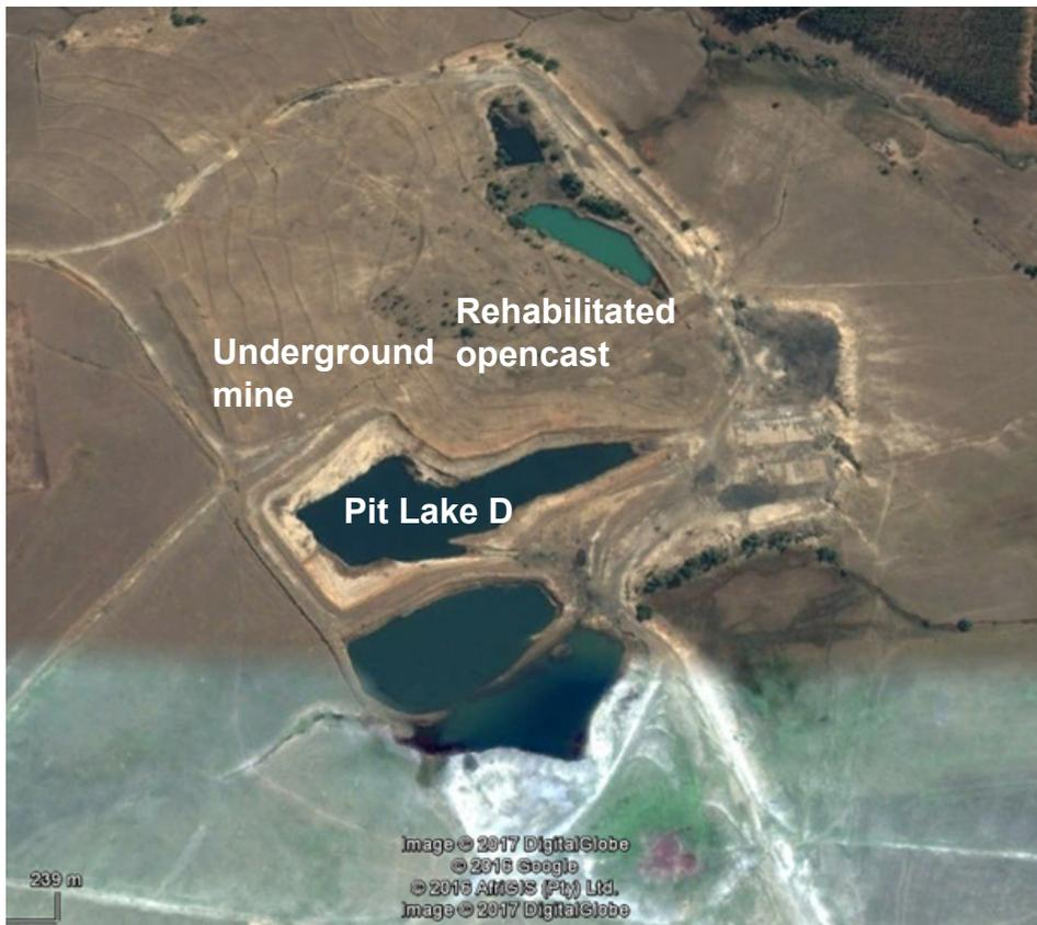
*Figure 10: Plan view of Pit Lake D indicating the underground portion and rehabilitated opencast area.*
