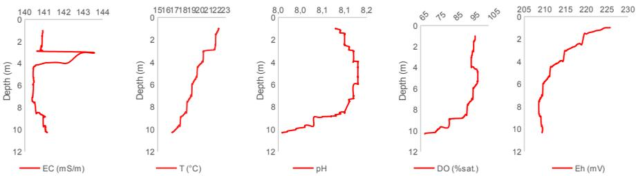
Figure 14: Water column profiles of Pit lake D (November 2016.)
