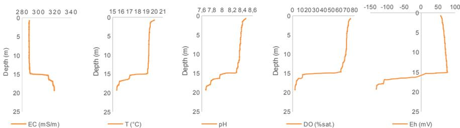
**Figure 12:** Water column profiles of Pit lake B (April 2017).
