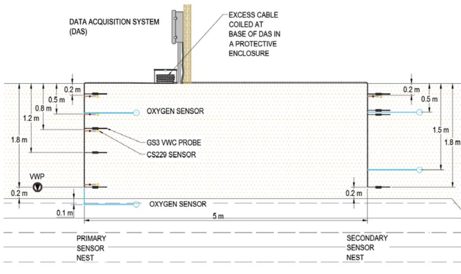
**Figure 2** Martabe WRSF sealing layer monitoring system.
