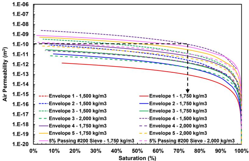
**Figure 6** Air permeability of Martabe material under various levels of compaction.
