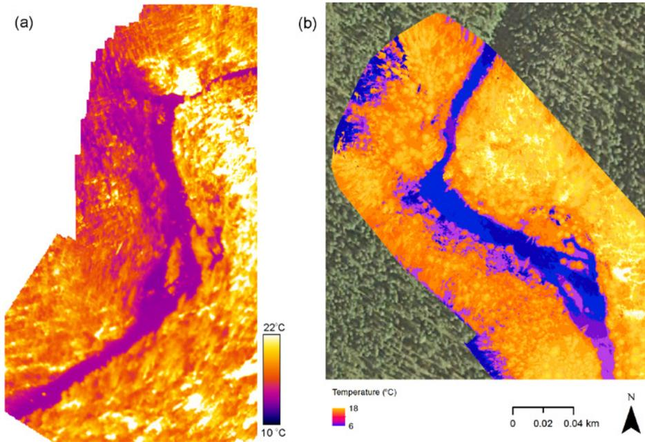
**Figure 4** TIR images with two acquisition methods: (a) helicopter and (b) UAV.
