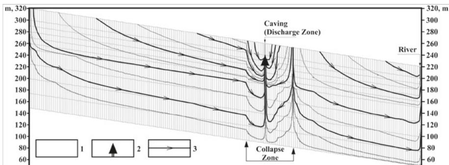
**Figure 2** The scheme of groundwater movement after flooding (on the left – the surface watershed, the impermeable boundary; to the right – the river; the size of the block horizontally – 50 m, the number of layers – 10). 1 – grid layout; 2 – groundwater discharge into the caving; 3 – the direction of groundwater flow.
