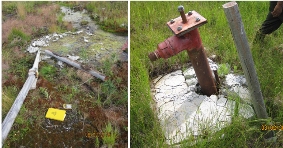
Figure 1 Artesian site. Artesian water welled up at a site with two markers (Site DDH 7380/7386) where the casing has been removed. Some casings, like DDH 8410 pictured with a base of cracked cement, had plugs or plates bolted to them, presumably to prevent artesian flow. A similar bolted casing was artesian through a broken ball valve.
