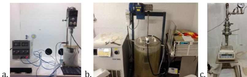
**Figure 1** a. EC reactor 1L b. EC reactor 70 L c. Nutsche filter.
