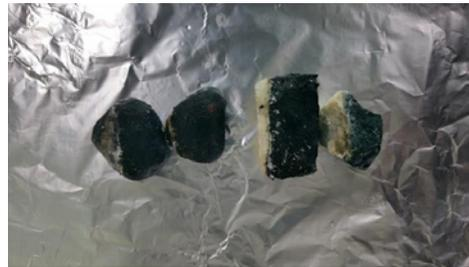
**Figure 1** (a) Mn removal reactors after 120 days (S, SL, SG, B and FA from left to right) and (b) Mn precipitates on the surface of Mn-coated gravel (left) and limestone (right) after reactor operation.
