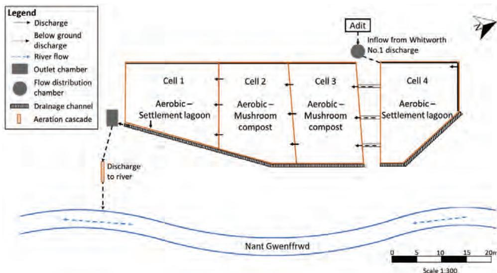
Figure 1 Schematic of Whitworth No.1 in 2017
