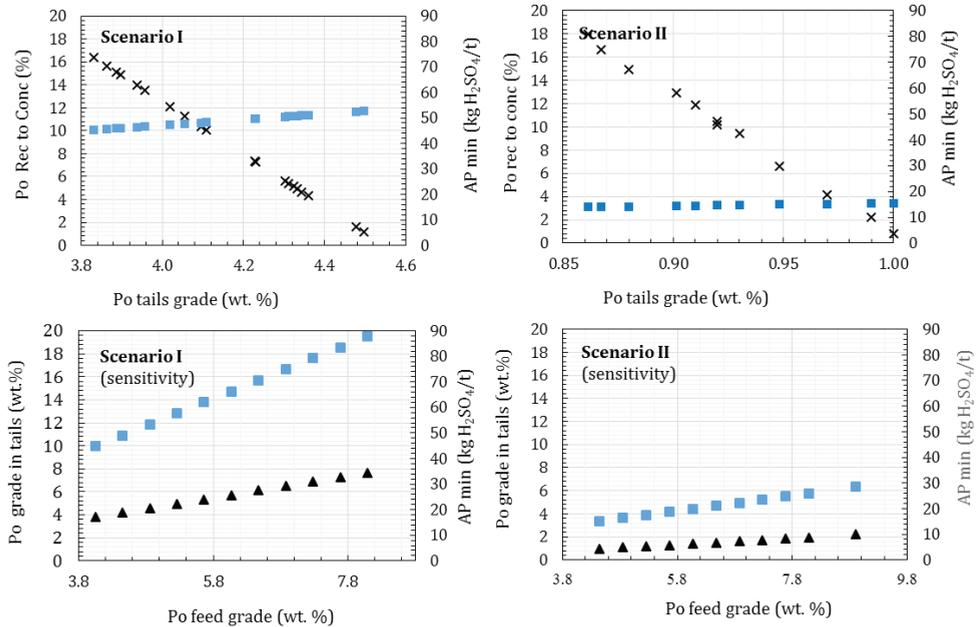
**Figure 3** Modelled AP min for the two scenarios analysed with their associated sensitivity analysis (see text for detail). □ indicates AP min, X indicates pyrrhotite (po) tails grade and Δ indicates pyrrhotite feed grade.
