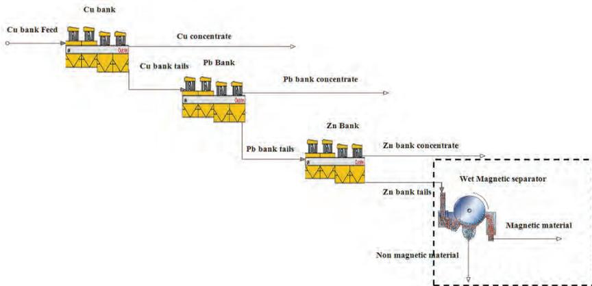
Figure 2 Flotation circuit configurations considered for the scenario analysis. Boxed inset illustrates the circuit modification for scenario II.
