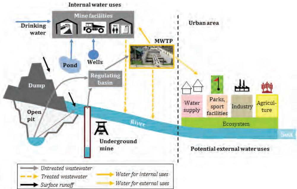
Figure 2 Conceptual model of the mine water management
