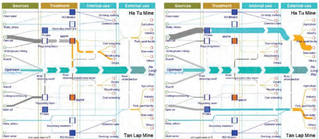
Figure 3 Material flow analysis of the water flow for the existing situation (left) and the final situation (right) (widths of arrows proportionally to flow quantity)
