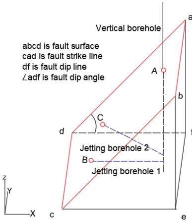
Fig.6 Fault detection based on radial jetting
