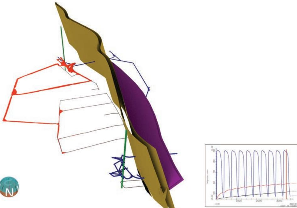
Figure 4 Calculated temperature field of the HT-MTES with temperatures coloured from red (high) to blue (low), regional fault system in yellow/violet (delta h)
