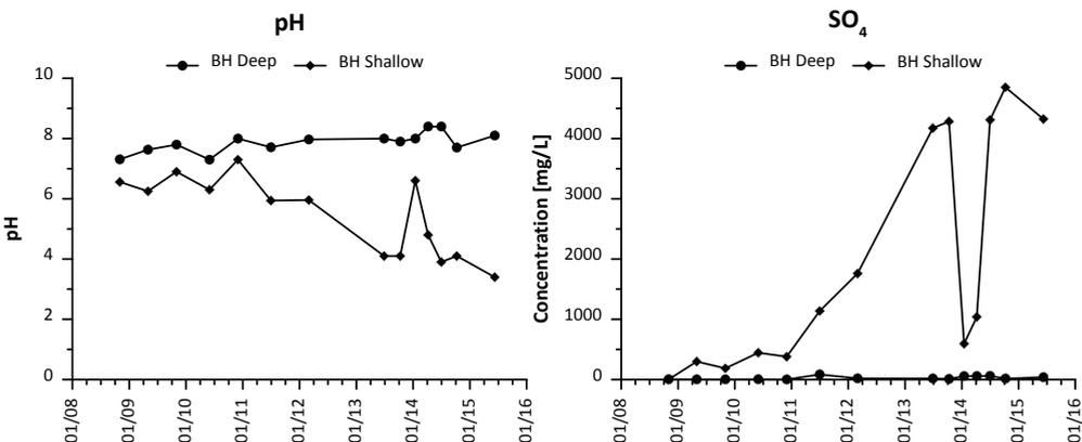
Figure 1 Groundwater quality monitored downstream of discard.
