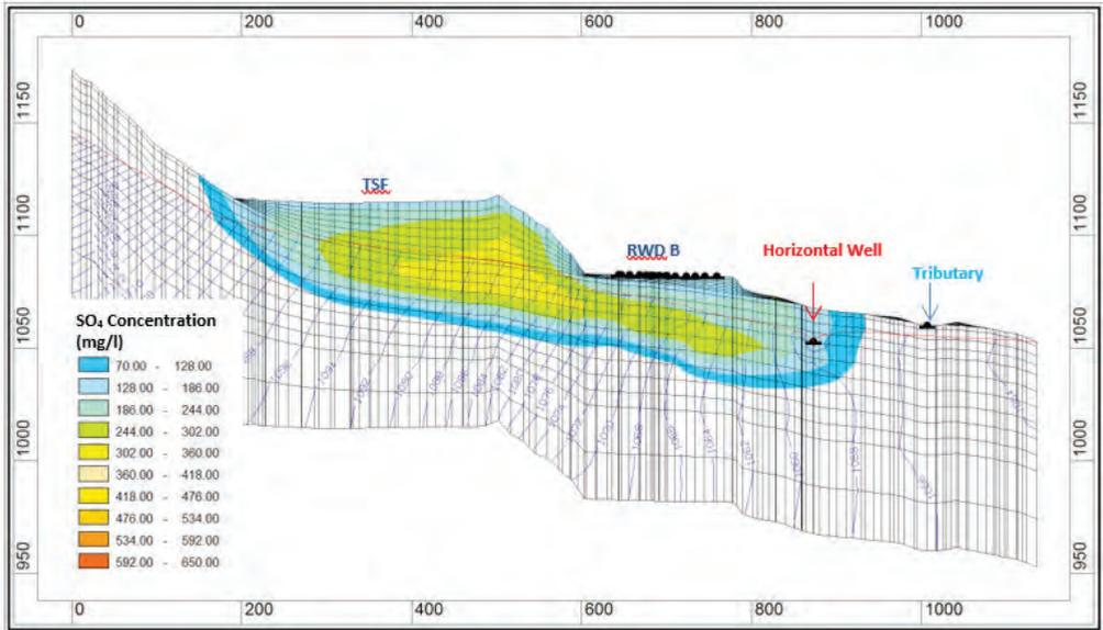
Figure 5 Cross section showing simulated plume extent 15 years after hydraulic plume containment using horizontal boreholes commenced.
