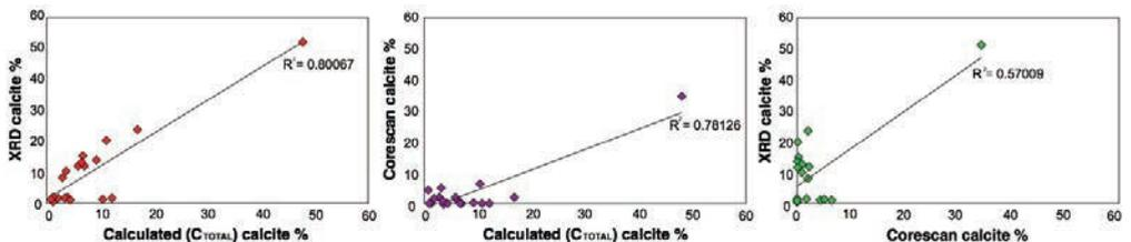
Figure 1 Comparison of calcite identification from XRD, Corescan<sup>®</sup> and calculated from total carbon values.
