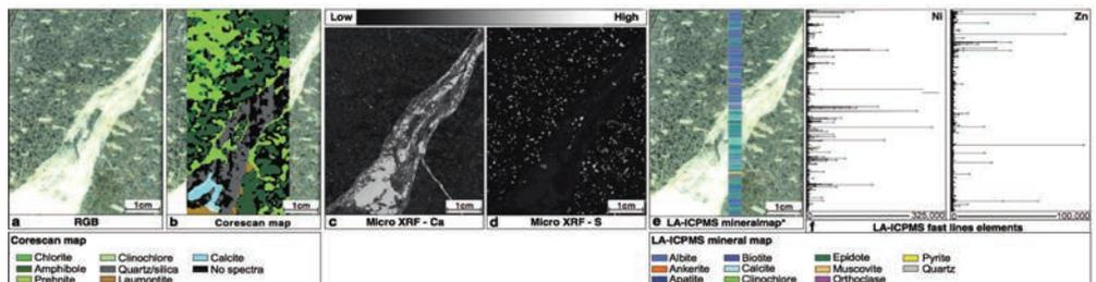
Figure 2 Drill core slab displaying mineralogy and trace element chemistry collected using different techniques; Corescan<sup>®</sup> classified mineral map, micro X-ray fluorescence ( $\mu$ XRF), mineral liberation analysis (MLA), laser ablation inductively coupled plasma mass spectroscopy (LA-ICP-MS) collected as fast line scans elemental data and derived mineralogy. \* LA-ICP-MS line not true line width to allow for visual representation.
