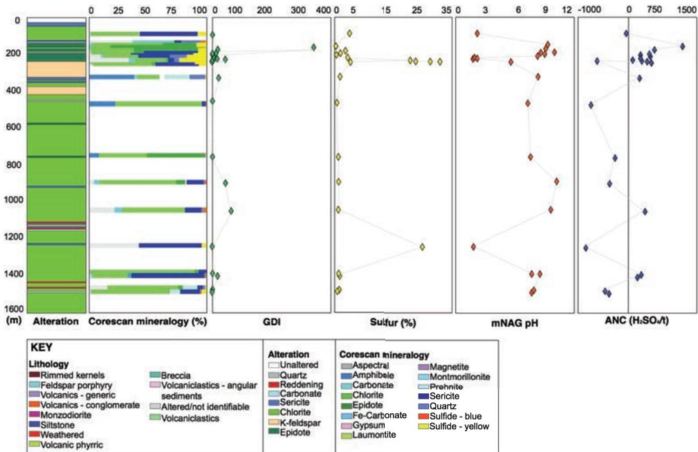
Figure 3 Down-hole log displaying lithology and alteration against Corescan® classified mineral map, geo-environmental domain index (GDI), sulfur %, paste pH, multi addition net acid generation (NAG) pH, acid neutralising capacity (ANC) and maximum potential acidity (MPA) value.
