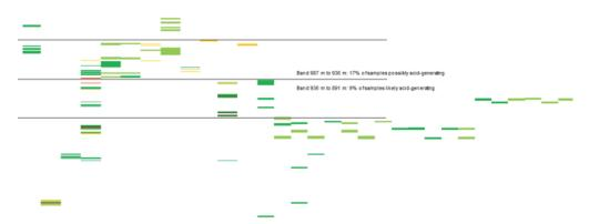
**Figure 5:** Example of thirty-one combined logs for a site, showing the occurrence of acid-generating material in a band, thick black lines showing top and bottom of transition zone, red for acid-generating material and green for non-acid generating material
