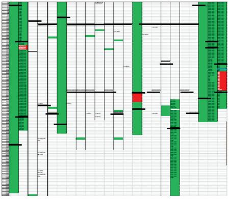
**Figure 4:** Example of twenty-three combined logs for a site, with observations arranged by depth (y-axis), thick black lines showing top and bottom of transition zone, red for acid-generating material and green for non-acid generating material
