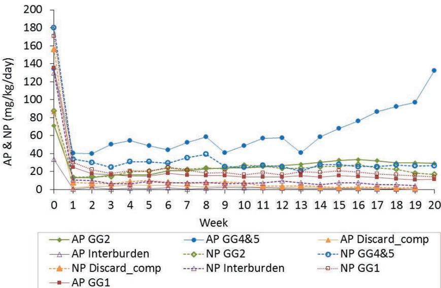
Figure 3 Kinetic results for coal discard material - Acid Potential and Neutralisation Potential (NP) vs time
