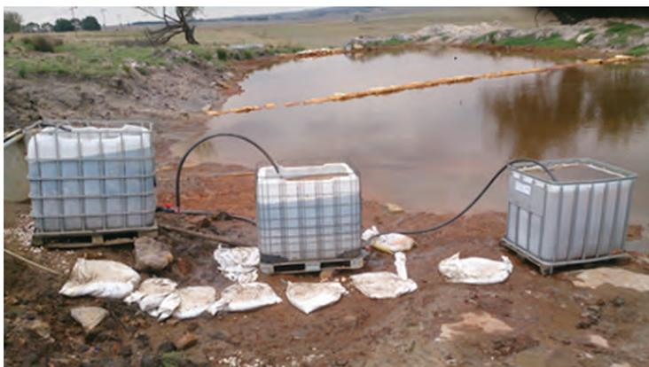
Figure 1 Carolina pilot passive treatment RAPS and oxidation units
