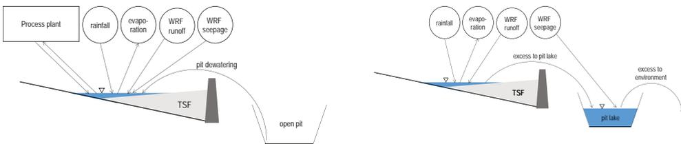
Figure 1 Schematic case study TSF water balance during operation (left) and after mine closure (right).
