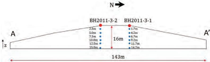
Figure 1 Cross-section schematic of the waste rock pile and the monitoring locations for internal pressure and pore-gas concentrations.
