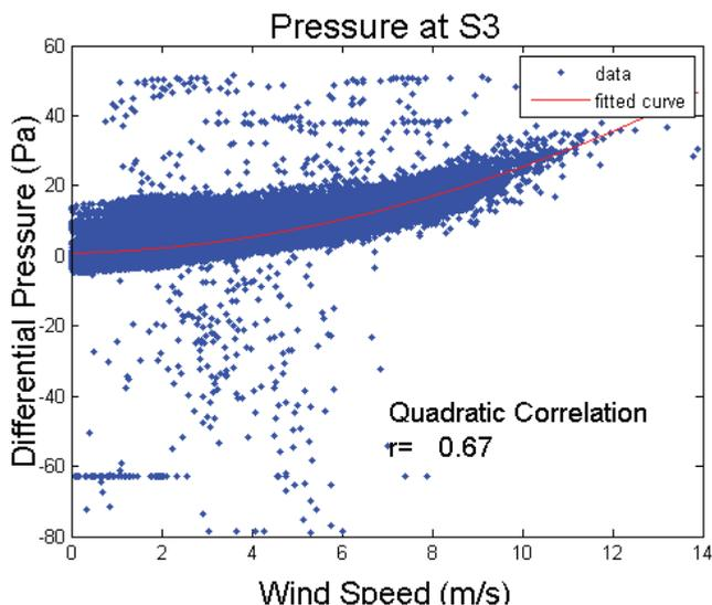
Figure 2 Correlation between wind speed and differential pressure at the southern toe.
