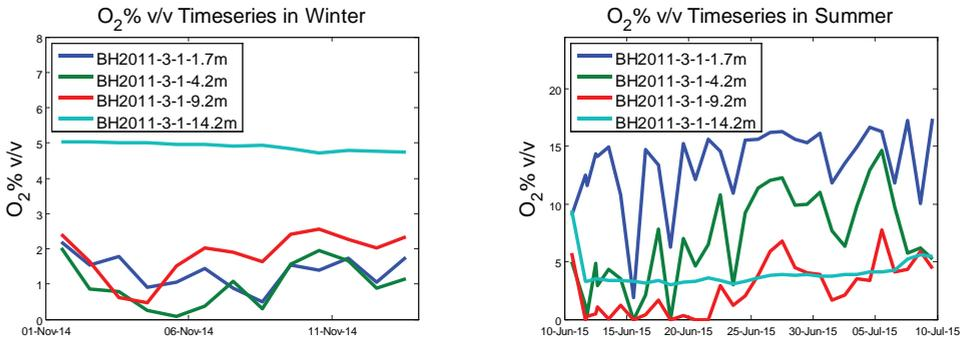
Figure 4 Time series for pore-gas oxygen content during a) a period in the winter and b) the summer.
