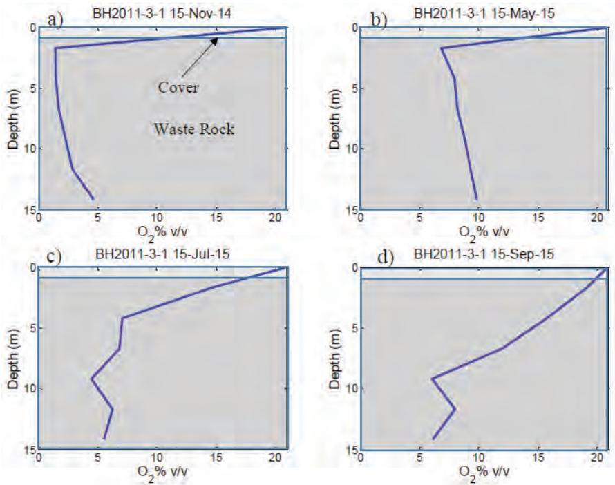
Figure 5 Pore-gas oxygen content with depth for a) typical diffusive profile during the winter on a) 15<sup>th</sup> November, 2014, b) 15<sup>th</sup> May, 2015, c) transition period including both the advective and diffusive profile on 15<sup>th</sup> July, 2015 and d) typical advective profile during the summer on 15<sup>th</sup> September, 2015
