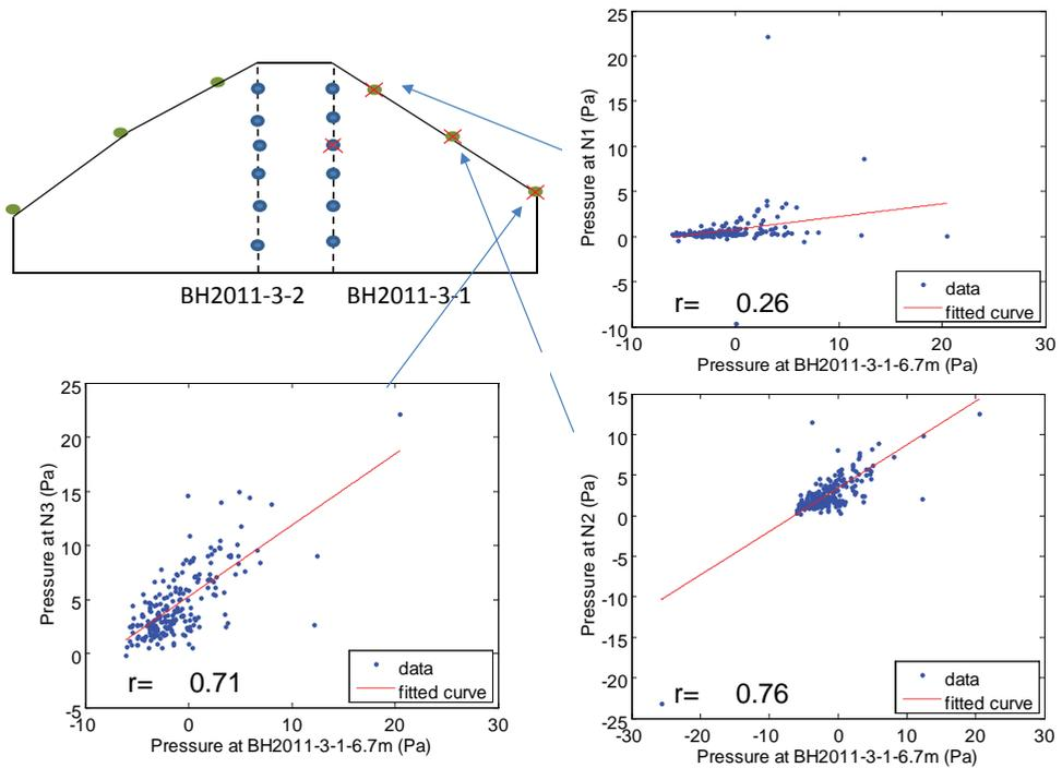
Figure 3 Correlation between the internal pressure at BH2011-3-1-4.2m and a) external location N1 (crest), b) external location N2 and c) external location N3 (toe). Daily averaged data sets. The data sets are predominately summer-time data but does include winter-time data as well.
