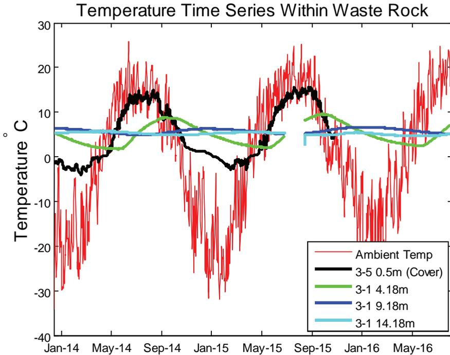
Figure 7 Time series for the ambient temperature and temperature within the cover and waste-rock at WRS#3.
