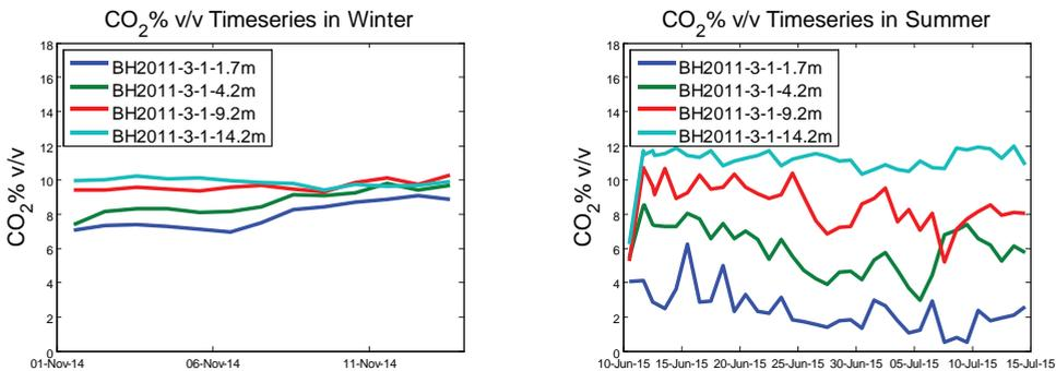
Figure 6 Time series for pore-gas carbon dioxide content during a) a period in the winter and b) the summer.
