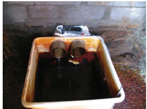
Figure 3 – Image of the ochre products in the study area. Crustification of surface drainage channels (left); Deposition of fluffy precipitates in the pipes, associated with the long term passage of the water (right).
