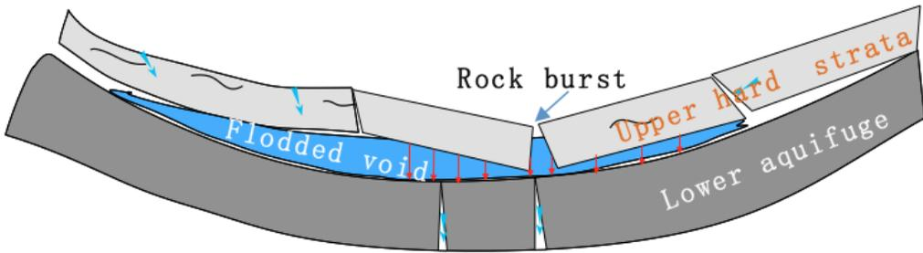
Figure 1 conceptual model of flooded sagging void.
