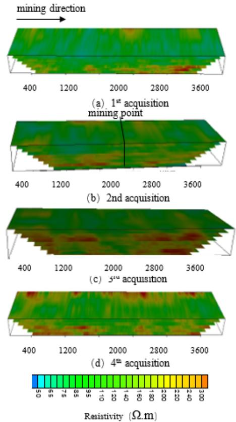
Figure 4 Resistivity slices of coal roof aquifer
