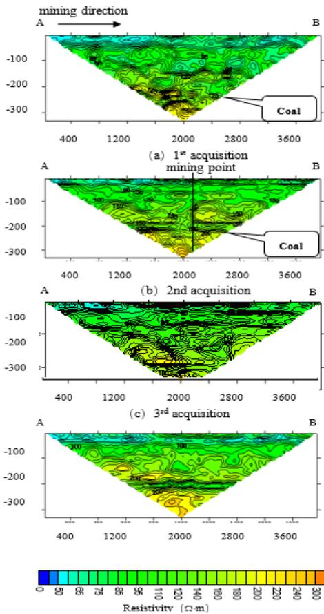
Figure 2 Geoelectrical I profiles comparison
