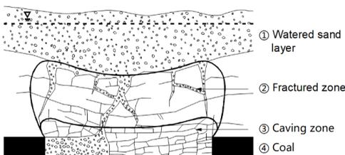
Figure 1 Diagrammatic sketch of quicksand through fractures
