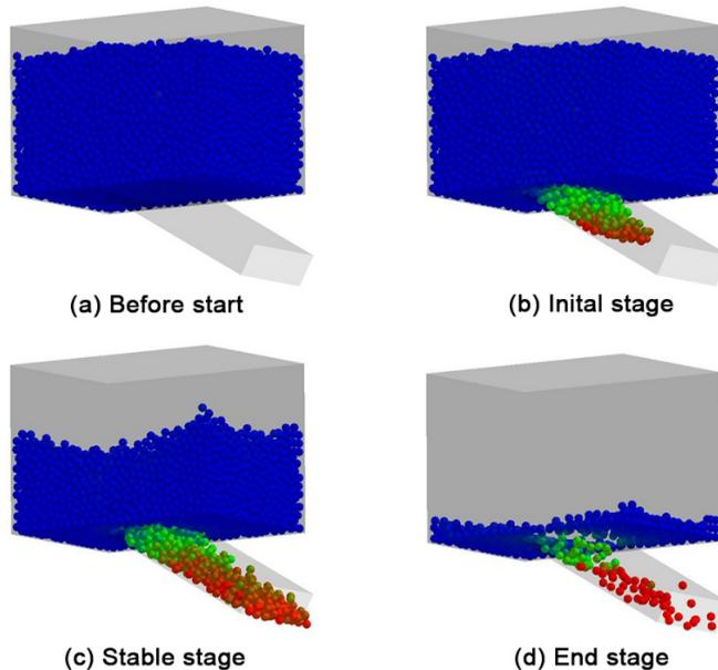
*Figure 3 Numerical simulation of water-sand mixture transport*
