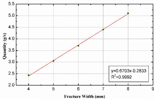
Figure 5 Mass flow rates of sand under different fracture apertures
