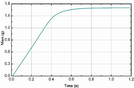
Figure 4 Curve of accumulative mass of sand versus time
