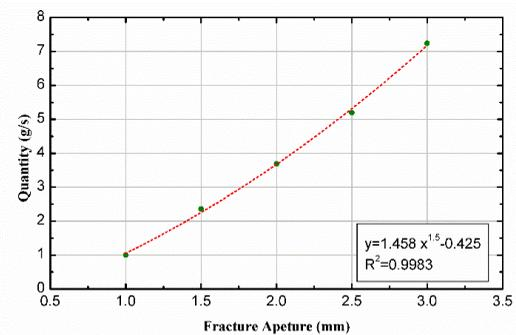
Figure 6 Mass flow rates of sand under different fracture apertures
