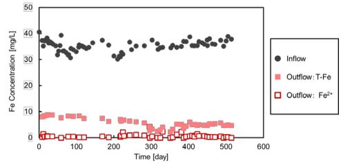
Figure 2 Changes in iron concentration of treated water
