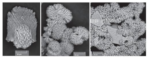
Figure 3 The morphology of calcite particles from a water sample: early rhombohedrons and late spherulites
