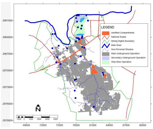
Figure 1 Site Layout map - blue circles represent borehole locations
