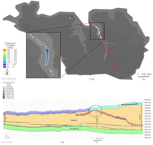
*Figure 7* Over pressurised areas within the pre-minind numerical model (plan view-top) – red dashed line indicates the cross-sectional line of the cross-section
