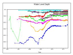
*Figure 4* Water level time graph of the shallow and intermediate groundwater regimes
