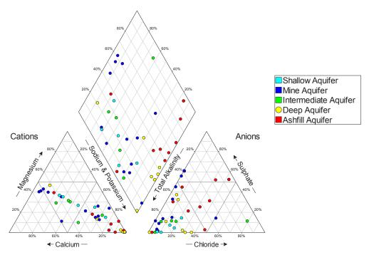
Figure 6 Expanded Durov diagram plot of the water qualities of all the groundwater regimes
