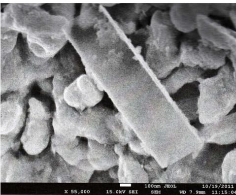
Figure 3 New formations on the surface of gold (nanofilm). Scale line is 100 nm
