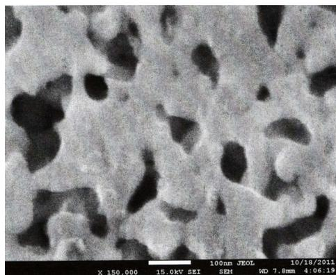
Figure 4 New formations on the surface of gold (nanopores). Scale line is 100 nm
