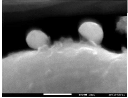
*Figure 6* New formations on the surface of gold (single particles of colloidal gold). Scale line is 100 nm
