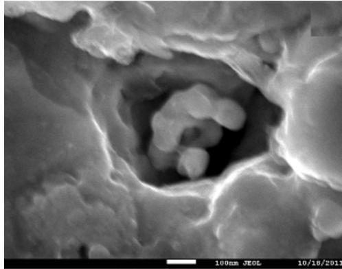
*Figure 7* New formations on the surface of gold (gold nanoparticles in the fossa). Scale line is 100 nm
