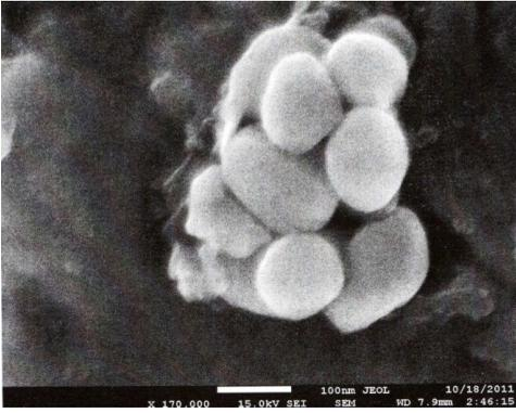
*Figure 5* New formations on the surface of gold (inclusions of micro- and nanoparticles of halite). Scale line is 100 nm
