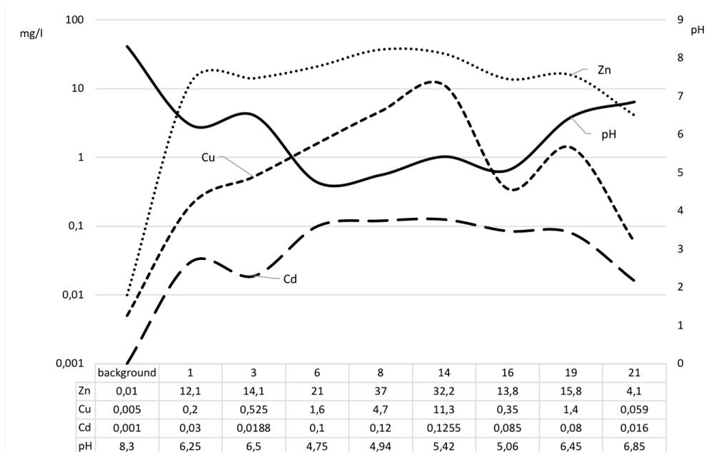
Figure 4 Changing of pH and PTM content in water along the Karagaily river (sampling points numbers are given in fig. 1)
