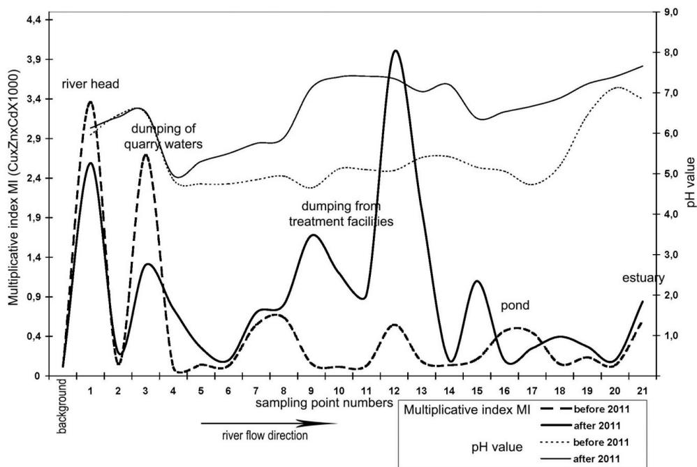
Figure 2 Changing of water pH and multiplicative index of Zn, Cu and Cd in bottom sediments along the Karagaily (Opekunov et al., 2018, revised and completed)
