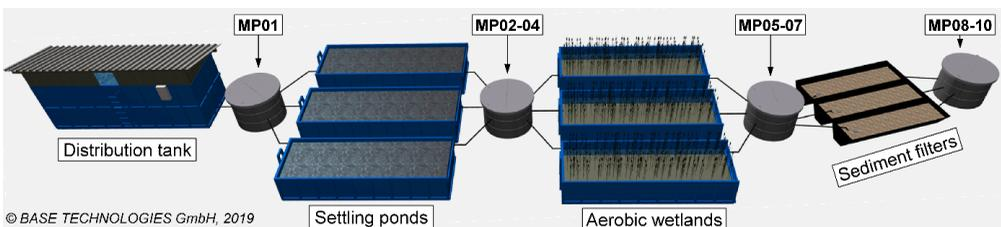
Figure 2 3D-illustration of the pilot plant (without terrain)
