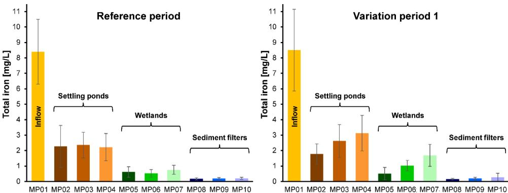
Figure 3 Iron monitoring in the pilot plant
