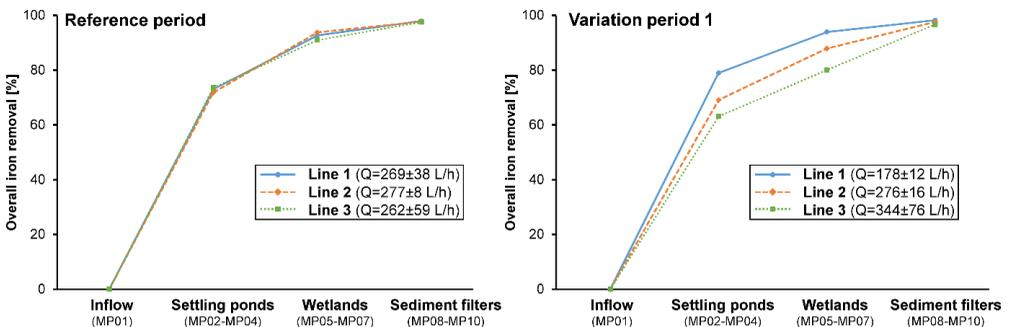
**Figure 4** Iron removal along the flow path with flow rates (Q)
