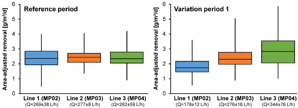
Figure 5 Area-adjusted removal in settling ponds with flow rates ( $Q$ )
