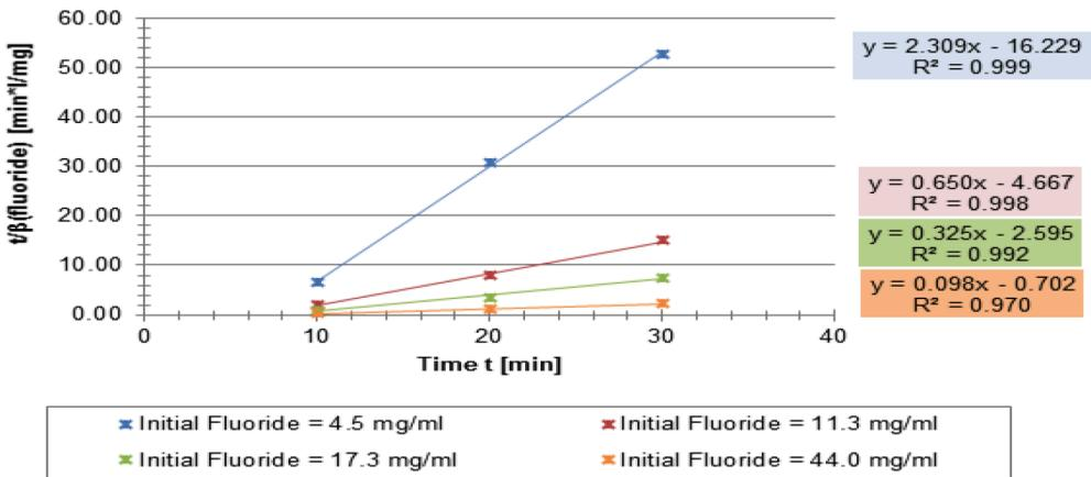
Figure 6 Applied Lagergren model for different initial fluoride concentrations
