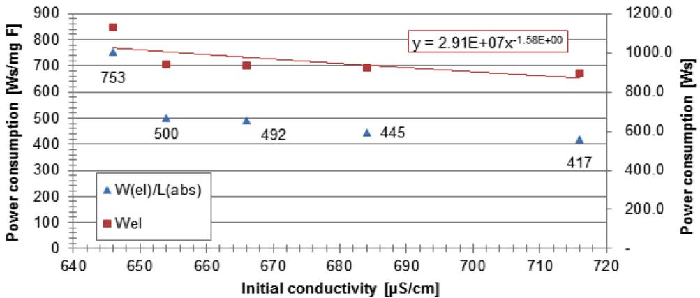
Figure 3 Power Consumption per Removed Amount of Fluoride at different Initial Conductivities
