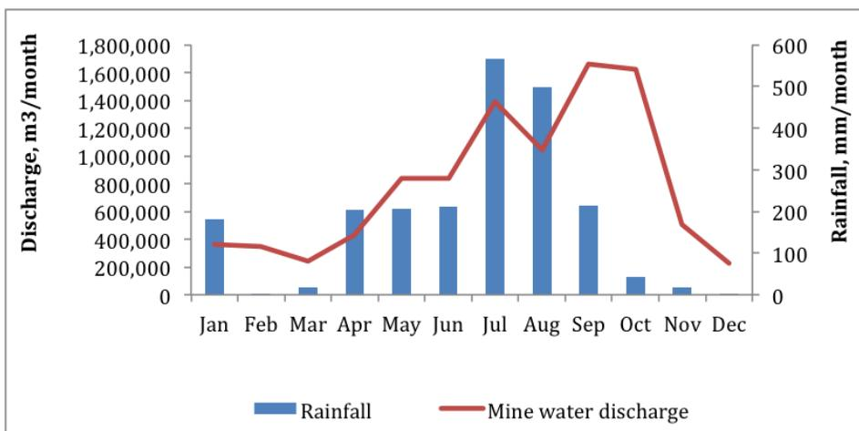
Figure 1 Diagram of the rainfall in Hon Gai area and the mine water drainage of Ha Tu O/P Coal Mine in 2016
