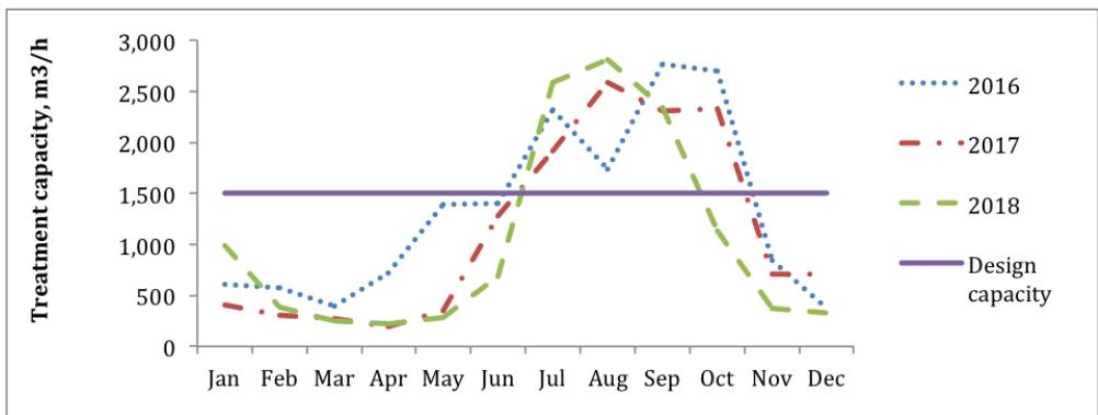
Figure 3 Development of treatment capacity of Ha Tu MWTP in 2016, 2017 and 2018
