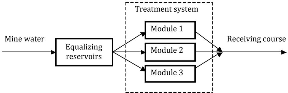
Figure 4 Principle of seasonal mine water management system
