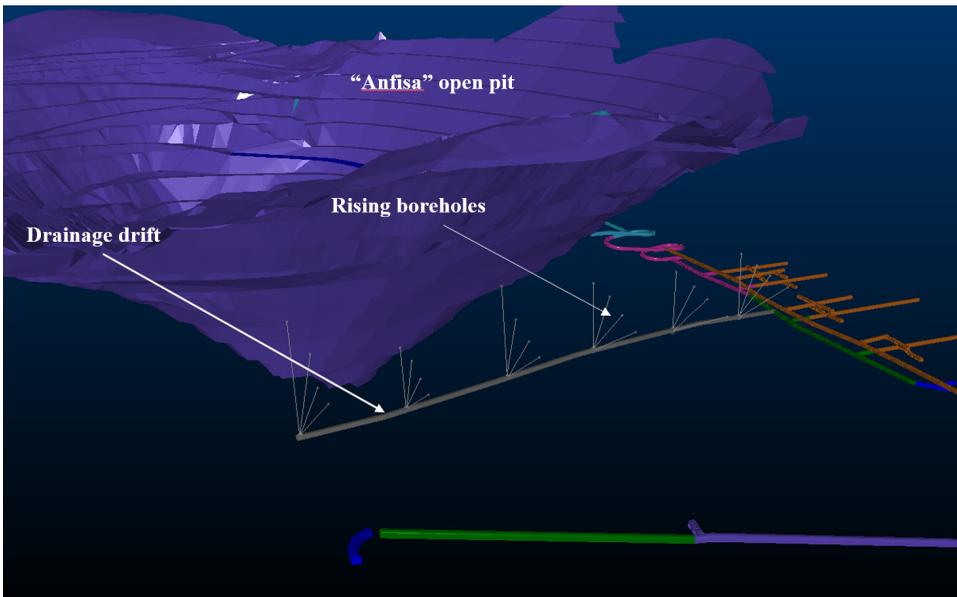
*Figure 4 3d model of the drainage drift with rising boreholes*
