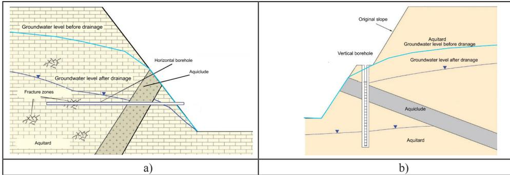
**Figure 2** Principal schematization of Horizontal (a) and vertical (b) boreholes use for drainage (Beale, G. and Read J., 2013)
