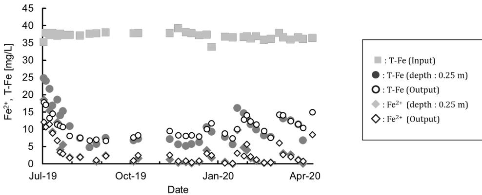
Figure 3 Annual processing performance of iron oxidation.
