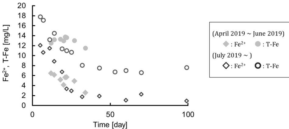
Figure 2 Changes in iron concentration of treated water.
