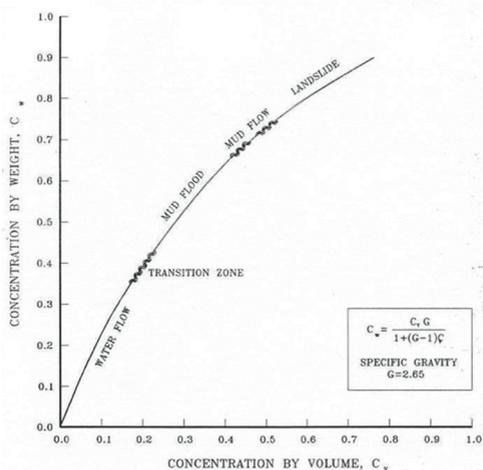
Figure 3 Flow classification based on sediment concentration (Flo2d-2012).
