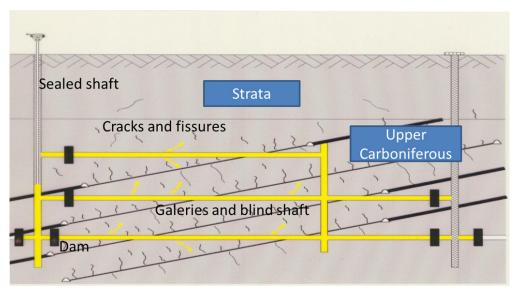
Figure 1 Schematic methane pathways to the surface (FZN).
